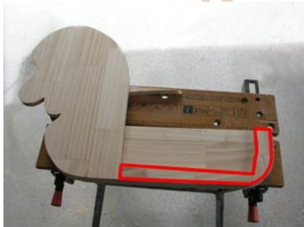
I used the offcuts, which must be the same thickness as the head, (marked in red in the photo) to make spacers for the body. Glue the spacers in place, and then glue the remaining body side in place, making sure that the top side where the seat fits is level. Sand the edges flush once the glue has set.
