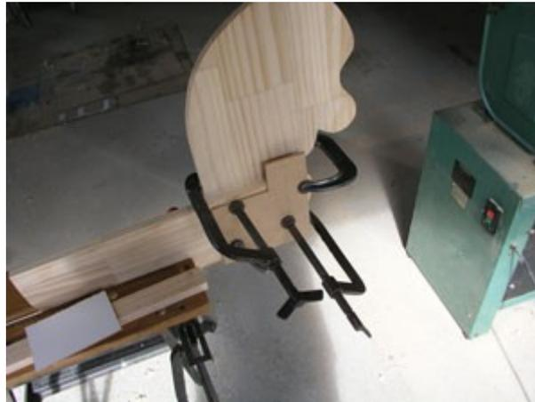
The photo above shows the head glued and clamped onto one half of the body.
