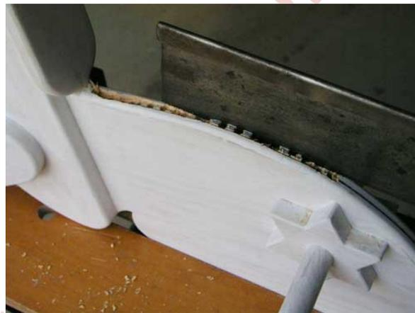
Using a tenon saw and a 6mm wide chisel, I cleaned up the groove as shown in the photo above. Using a router and round over bit, round off the edges except where it is attached to the body.
