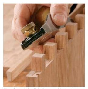
Chamfer and kerf the tenons. Saw the tenons like the dovetail pins. Before glue-up, use a block plane to lightly chamfer the ends (above) and then cut slots for wedges using a backsaw. Work-
