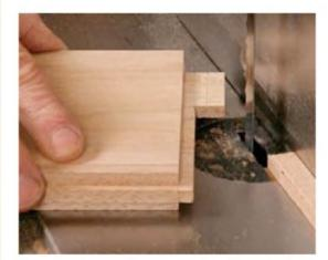
**Easy tongue-and-tenon combo.** Use a dado set to rabbet both faces of the panels to create a centered tenon. Then trim the tenons on the bandsaw as shown to leave a perfect throughtenon.
