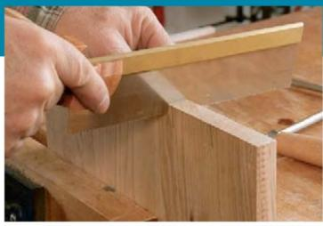
**Tails first, of course.** After scribing the baselines with a marking gauge, lay out the tails with a bevel gauge set to a 1:8 slope (left). Saw to the baseline with a backsaw (right). Don't worry about following your pencil line precisely; you'll scribe the pins to fit later. Just keep your sawcuts square and try not to go past the baseline.
