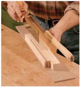
**Simple storage for saws.** Pekovich cut kerfs in pine blocks to secure his handsaws, scrapers, and combo square. The blocks are glued to an MDF base and installed as a single unit.
