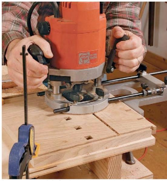
**Rout the grooves on the inside face.** Set the bit slightly deeper than the tongues on the panels to allow for glue squeeze-out. Cut the grooves along the edges of the sides before resetting the fence to cut the narrow dado for the drawer divider. You'll need to groove the well bottom, too.
