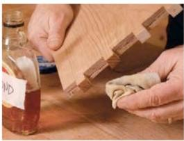
**Surface and seal.** The soft butternut planes easily and yields a shimmering luster (top). Apply a washcoat of shellac to all the parts, especially the end grain of the tenons and dovetails, but stay clear of the glue areas.
