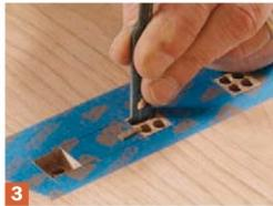
**Layout tip for old eyes.** Wood grain can make scribed lines tough to see, so Pekovich puts painter's tape on each face before marking the mortises. Use a marking gauge to scribe both the mortises on the sides (1) and the tenons on the shelf. Then use a square and marking knife to scribe the top and bottom edge of the mortises (2). Peeling away the tape provides a clear border for drilling out the waste and chopping the mortises square (3). Work inward from both faces.
