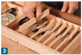
No-math solution for dividers. Start by milling divider stock to match the width of a \*/-in. dado stack. Then set your tools where you want them and mark dado locations wherever you need a divider (1). Cut dadoes for the dividers in pairs (2). Install the dividers, making cutouts to allow easy access to your tools (3).
