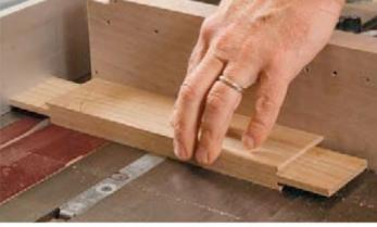
**Tenons last.** Align the blade with the outside of the panel groove to cut the tenon cheeks (left). To cut the shoulders, trim away most of the waste first on the bandsaw to avoid a trapped offcut, and then use your miter gauge and rip fence (above) for the final cut.
