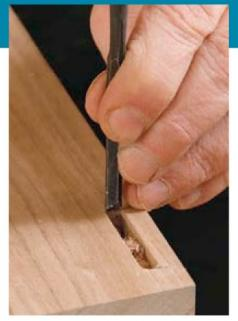
Little through-tenons first. Start these on the outside face. Use a router with
