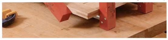
Clamp from three directions. A bridle joint needs a lot of help to pull it together. Start by clamping across the rails, then add clamps across the stiles (left). Check to make sure that the joints are pulling closed in each direction as you tighten the clamps. Finally, clamp vertically at each corner to ensure a good glue bond (above).
