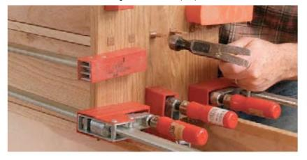
stress and avoid any surprises once the glue is on. For the actual glue-up, use plenty of clamps to bring the case together. Then put glue in the slots in the shelf tenons and drive wedges in place (left).
