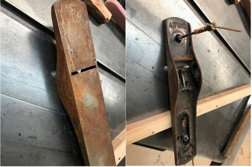
The base of the plane is very rusty. I will need to assure a solid electrical connection to the metal, however. In this case I can use one of the handle screw posts to wrap a section of copper wire around for that purpose.
