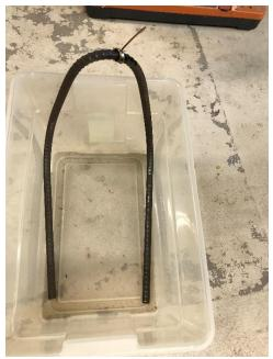
This section of rebar was bent to fit the tub I am using and the middle section will remain above the electrolyte. I soldered a short section of copper wire to the rebar to assure a good electrical connection, but that is probably overkill.
