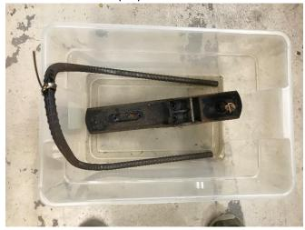
Make sure the object being de-rusted and the sacrificial electrode can remain in a position where they do not touch since that will short-circuit the voltage source.
