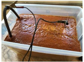
As the process progresses, you will see the rusty brown foam accumulate on the surface of the electrolyte. This is normal. Once the bubbles stop forming, the process is complete. Turn off the voltage
