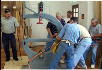
is now in service. This is a rather unique saw - it is a 36" saw with approximately 13" re-saw capability. It was built in the late 1800's and originally designed to be driven by a steam engine. The bearings for the upper and lower wheels have cups that you fill with sawdust and then saturate with oil in order to provide lubrication. We owe a big thanks to **Charlie Ard** and **John Lawson** for
