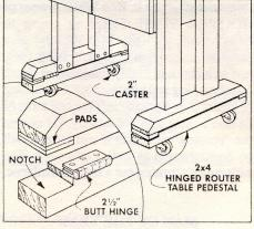
I designed a simple "flip-down" system that works great on my router table and could be adapted to other machines. I mounted 2" casters to two pieces of 2x4 and then hinged the 2x4's to the pedestals of the router table. When the table is in use the casters are kicked inward and the feet rest firmly on the ground.
