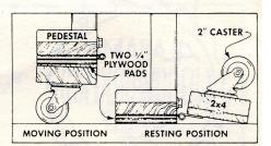
Before the 2x4's are mounted, wide notches are cut on both ends. This allows the 2x4's to clear the pedestal pads when they're flipped into position.
