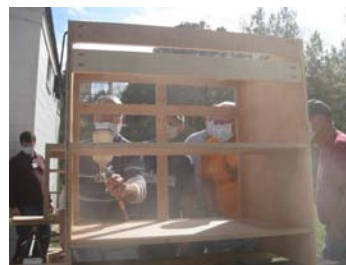
Dan Browning demonstrates his technique for spraying sanding sealer.
