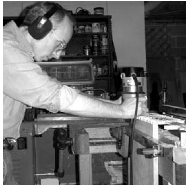
Marty cutting dovetails on his cherry blanket chest during the Blanket Chest Class
