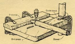
serve as a length stop. Lower the quill to take a light cut, lock the quill in place and rotate the dowel under the bit. Continue taking light cuts until you're at the desired diameter.
